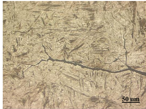
Figure 11 Same sample as Fig. 9 showing random orientation of the crack path. No Ni-rich phases are present in the microstructure.
